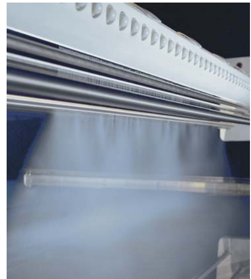
Fig 3: Lubricating aggregates: Roll lubrication (top left) [5], Spray lubrication (bottom left) [5], Electrostatic lubrication with an inline hotmelt device (top right) and electrostatic lubrication by means of atomised spray (bottom right)
